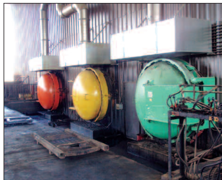
...and treated either with creosote alone or with a dual borate/creosote process
